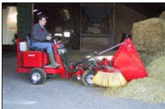
Figures 1 and 2. “Clean Girl” sweeps stall beds, applies bedding, and scrapes or sweeps manure away from the stall curb while the operator drives the machine.
