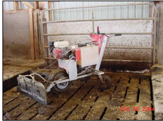
Figure 4. “Choremate” is a walk-behind, self-propelled scraper manufactured in Ingersol and sold by Performance Dairy Centre, Embro, ON, Telephone: 1-519-423-9119.
