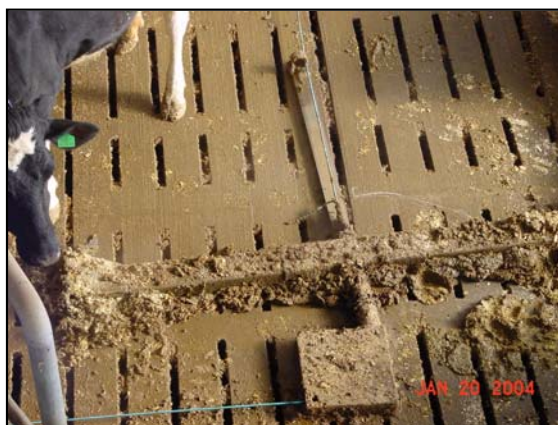
Figure 3. Cleaning slatted floors is a way to improve foot cleanliness and decrease contamination of beds. The photo shows an alley scraper in operation on slatted floors in a new Ontario dairy barn.
