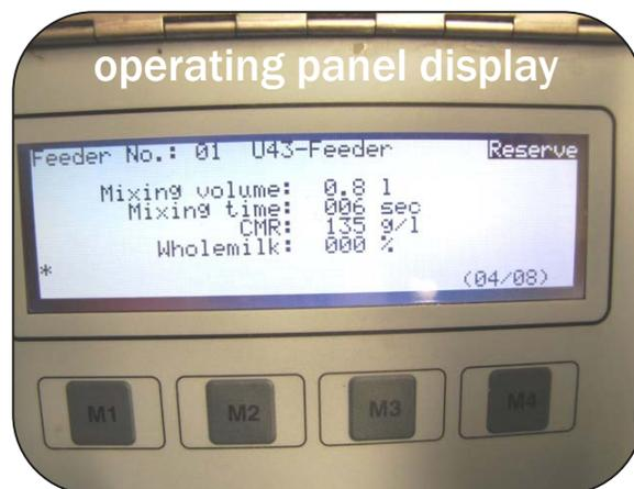
**Figure 2.** Record the data from the operating panel display to show what the machine is programmed to do.
