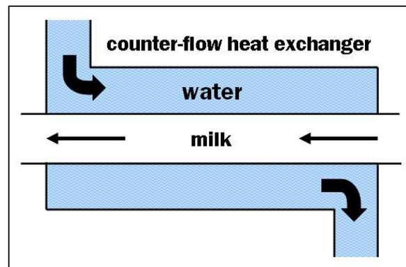
**Figure 1. A counter-flow heat exchanger.**
