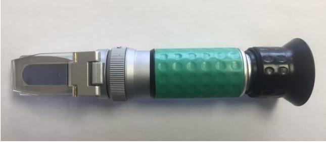
Figure 2. A manual refractometer such as this one can be used to measure total solids content of colostrum
